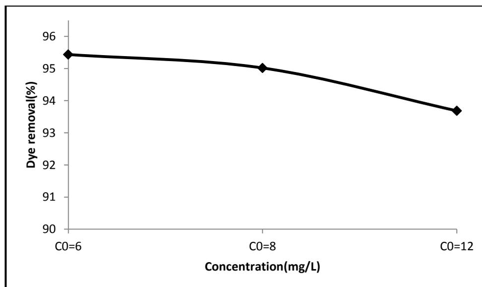
**Figure 2.** Effect of different dye concentrations on dye removal by Copper oxide Nano-particles; pH 2, 25 °C, agitation rate of 180 rpm and 0.233 g adsorbent in 50 ml of dye solution.
