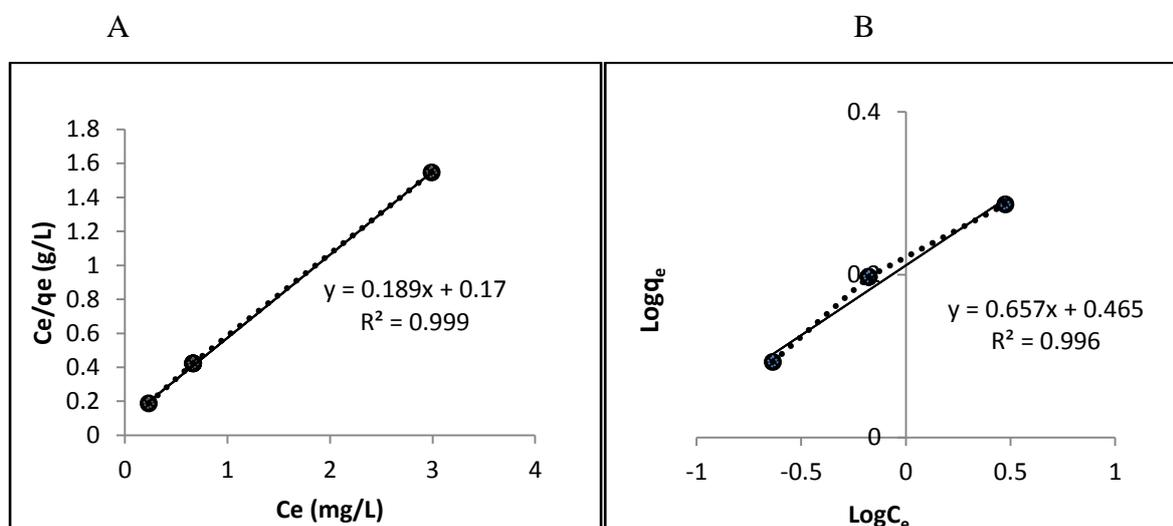
**Figure 5.** Langmuir (A) and Freundlich (B) isotherm plot for Erythrosine dye adsorption on Copper oxide nano particles.
