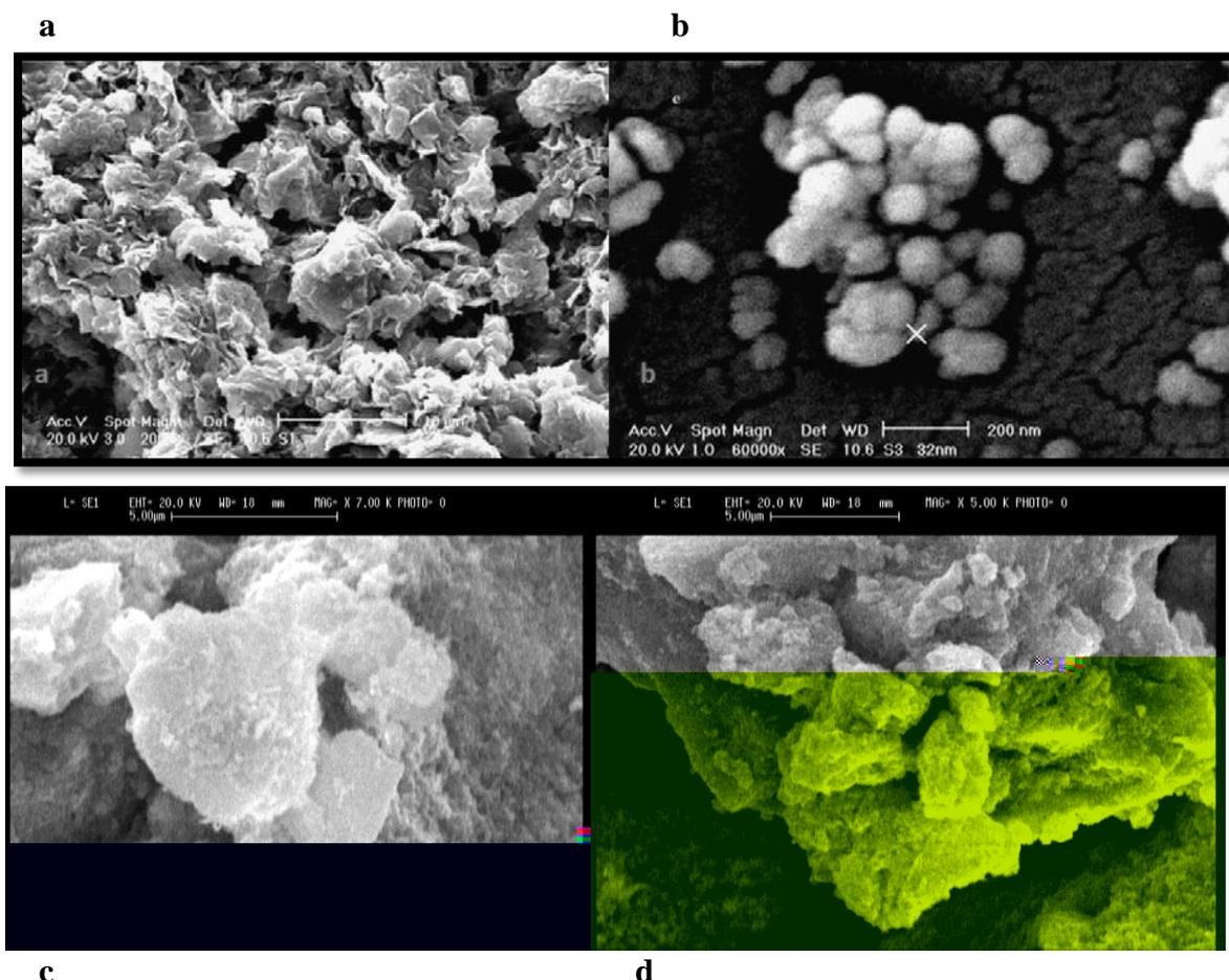
**Fig.7.** Scanning electron micrographs of (a) original CuO nano particles, (b,c,d) dye adsorbed CuO nano particles with Erythrosine. conditions: pH 2, 0.233 g in 50 ml of adsorbent, 12 mg L<sup>-1</sup> of initial dye concentration, equilibrium time of 90 min, agitation rate of 180 rpm, 25 ± 1 °C and particle size of 32 nm.
