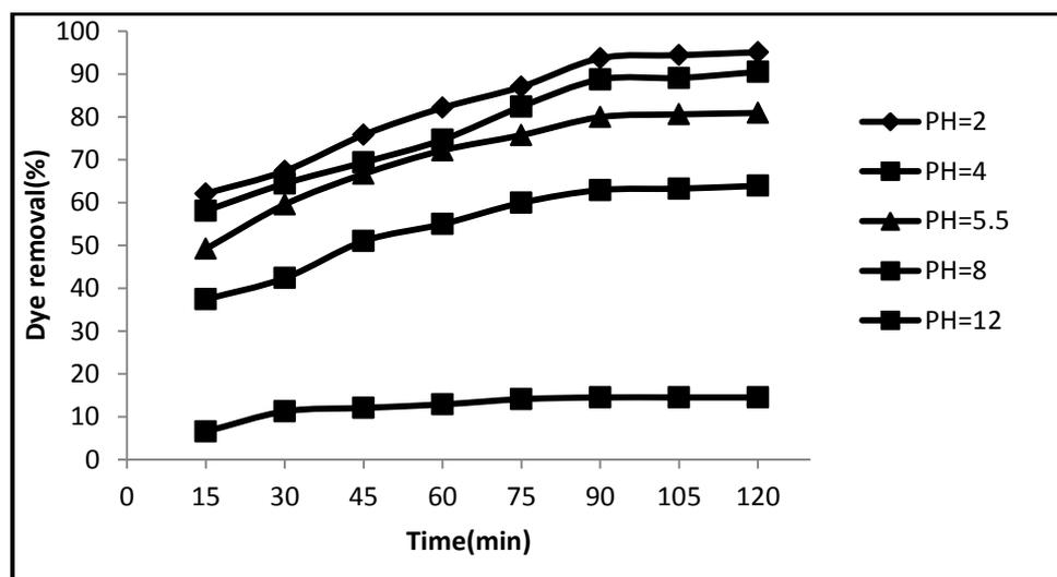
**Figure 4.** Effect of pH different time on the removal of Erythrosine; 90 min contact time, 25 °C, agitation rate of 180rpm and 0.233 gr adsorbent in 50 ml of 12 mg L<sup>-1</sup> dye solution.
