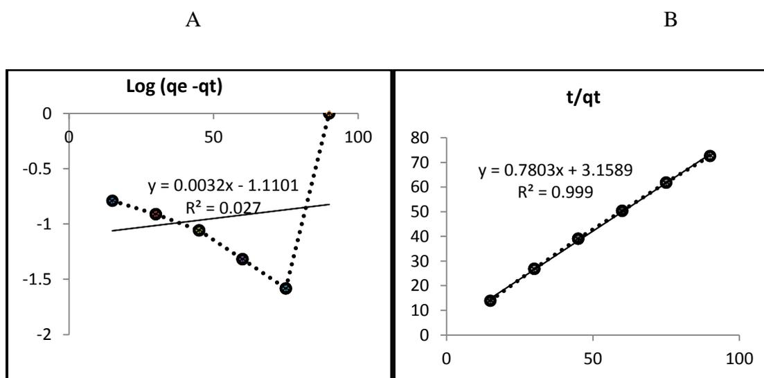
**Fig. 6.** Pseudo first order (A) and Pseudo second-order (B) adsorption kinetics of Erythrosine dye onto Copper oxide nanoparticles; pH 2, 25 °C, Initial dye conc. of 6 mg L<sup>-1</sup> and rate of 180 rpm.
