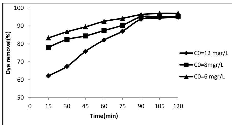
**Figure 1.** Effect of contact time for different dye concentrations on dye removal by Copper oxide nano particles; pH 2, 25 °C, agitation rate of 180 rpm and 0.233 g adsorbent in 50 ml of dye solution.
