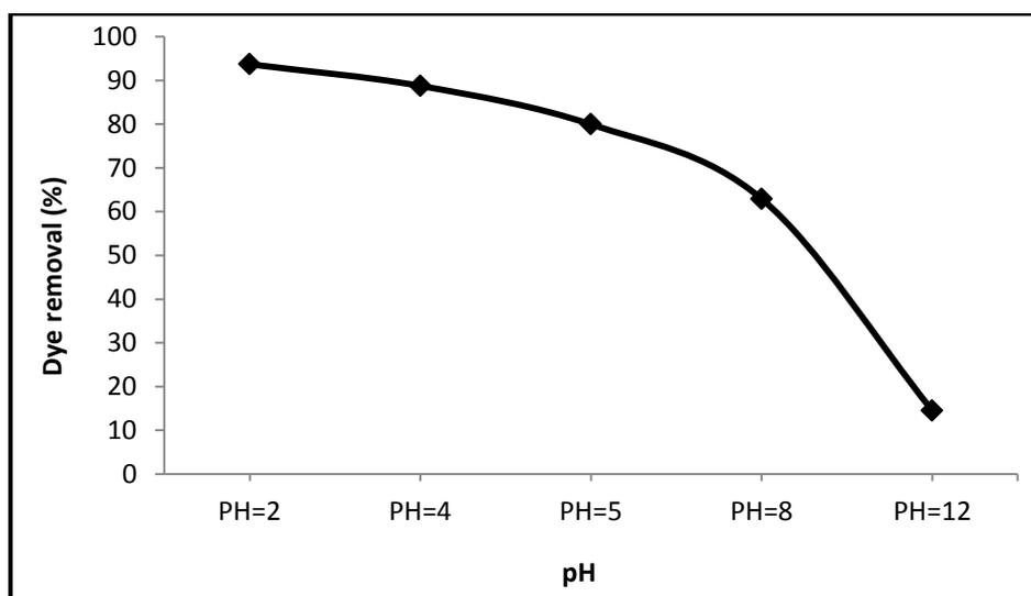
**Figure 3.** Effect of pH on the removal of Erythrosine; 25 °C, agitation rate of 180rpm and 0.233 gr adsorbent in 50 ml of 12 mg L<sup>-1</sup> dye solution.
