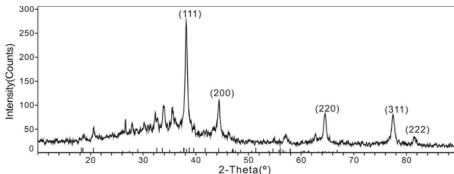
**Fig 2.** XRD pattern of the TiO<sub>2</sub> nanoparticles
