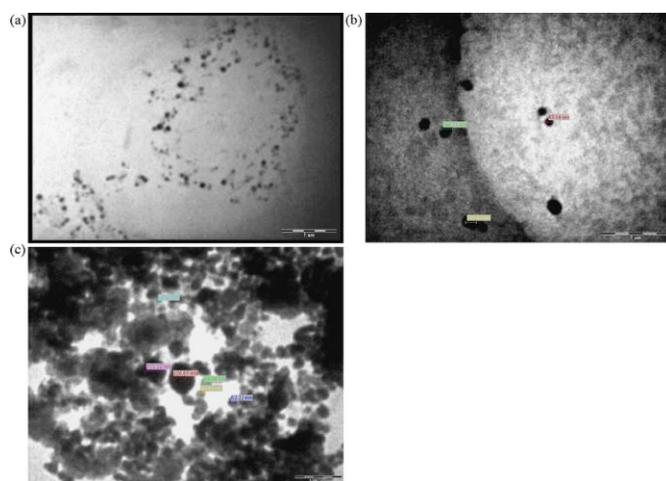
**Fig.1.**TEM imTiO<sub>2</sub> of (a)synthesized colloidal silver nanoparticle, (b) the TiO<sub>2</sub> nanoparticles immobilized on silica gel (c) TiO<sub>2</sub> grafted silver nanoparticle
