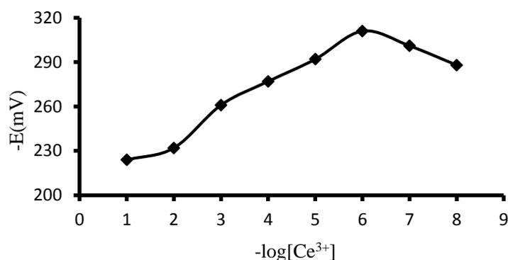
**Figure 2.** Calibration curve of the  $\text{Ce}^{3+}$  selective sensor based on kryptofix22DD.
