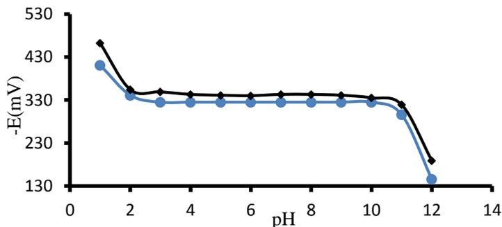
**Figure 5.** Effect of the pH of test solutions on potential response of the  $\text{Ce}^{3+}$  selective sensor (●  $1.0 \times 10^{-3}$  M, ◆  $1.0 \times 10^{-4}$  M).
