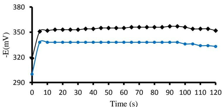
**Figure 3.** Static response time curves of the  $\text{Ce}^{3+}$  selective sensor ( $\bullet$   $1.0 \times 10^{-3}$  M,  $\blacklozenge$   $1.0 \times 10^{-4}$  M).
