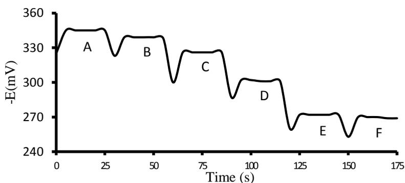
**Figure 4.** Dynamic response time of the  $\text{Ce}^{3+}$  selective sensor for step changes in the concentration of  $\text{Ce}^{3+}$ : (A)  $1.0 \times 10^{-6}$  M, (B)  $1.0 \times 10^{-5}$  M, (C)  $1.0 \times 10^{-4}$  M, (D)  $1.0 \times 10^{-3}$  M, (E)  $1.0 \times 10^{-2}$  M, (F)  $1.0 \times 10^{-1}$  M.
