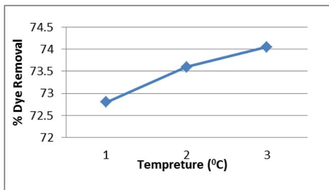
Fig (11): Effect of different temperature on removal of erythrosine pH 4, 25 °C, agitation rate of 180 rpm and initial dye concentration 8 mg L<sup>-1</sup> in 150 ml of dye solution.
