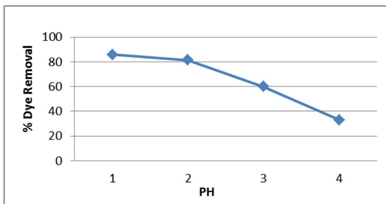
**Fig 3.**Effect of pH on the removal of erythrosine 25 °C, agitation rate of 1800rpm 0.733 gr adsorbent in 100 ml of 8 mg L<sup>-1</sup> dye solution
